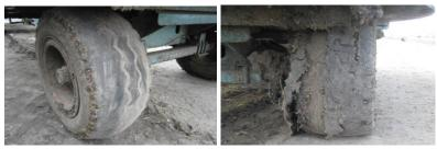
Fig. 1. Wear of the forage mixer wheel tread
