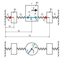
Fig. 5. Dynamic model of the mobile combined forage preparation unit with the improved working body
