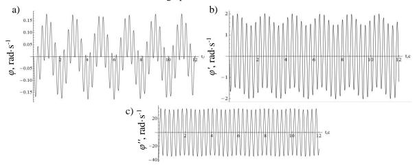
Fig. 4. **Results of the research of dynamics of work of the mobile mixer:** a – schedule of the change of angular movement; b – graph of changes in angular velocity; c – schedule of the change of angular acceleration
