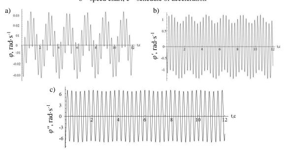
Fig. 7. Results of the study of dynamics of the mobile feed preparation unit: a – schedule of changes in angular displacement; b – graph of changes in angular velocity; c – schedule of changes of angular acceleration
